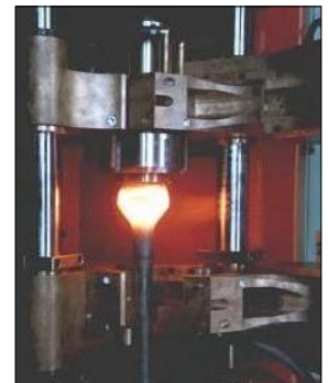
Upsetting in progress
