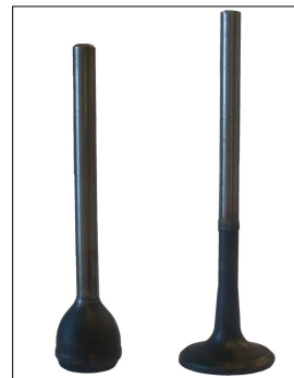
Example upset engine valves. Before stamping / after stamping
