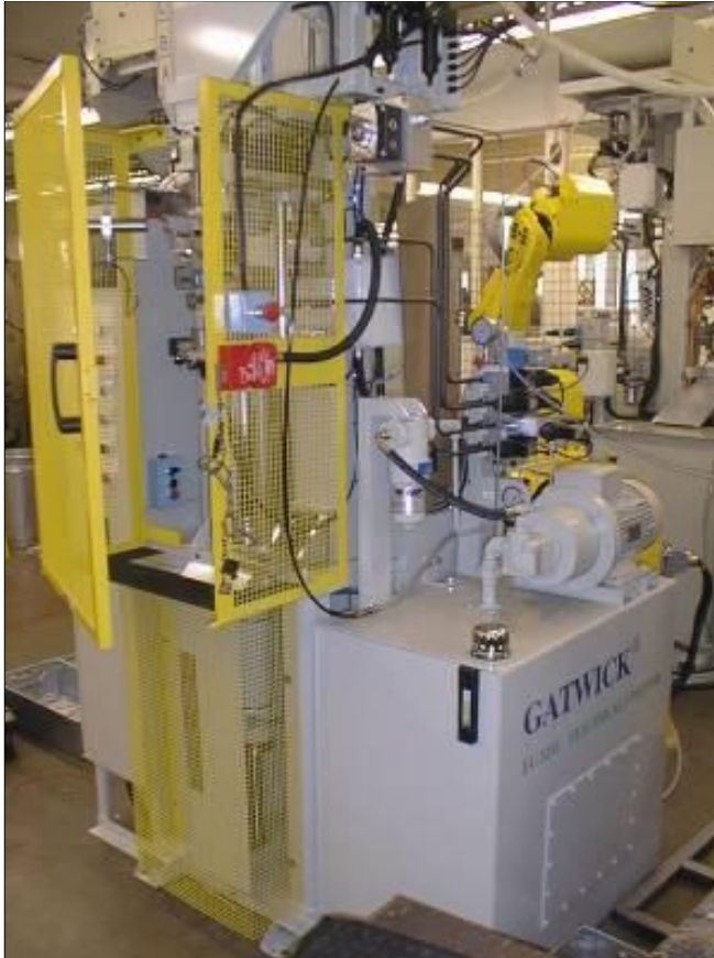
EUM32 with automatic part feeding and robotic removal of welded components
